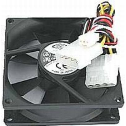
radiate away inside the computer's case. Adding a fan greatly increases the efficiency of the heatsink, and is the perfect way to help combat an overheating CPU.
