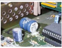
PCB. Clean off all traces of gunk as outlined above. The Amiga will continue to function with the exception that the clock will need to be set each time on power-up.
