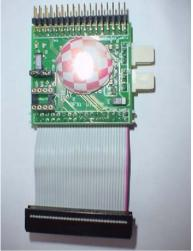
Pictured above is the prototype of the DFX floppy interface for std pc floppy drives. It allows the reading and writing of Amiga std and high density floppys with a PC floppy drive.
